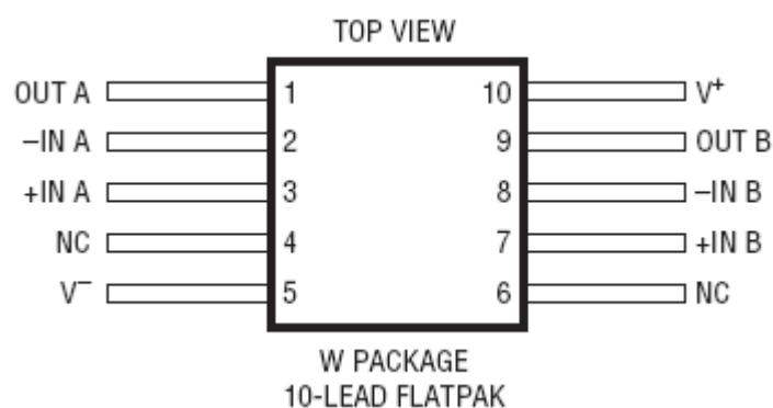
Figure B.2. W package drawing (for reference only). This figure was extracted from the LINEAR TECHNOLOGY CORPORATION RH1498M Datasheet.
