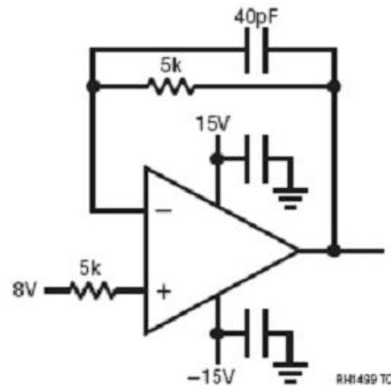
Figure B.1. Irradiation bias drawing for the units to be irradiated under electrical bias. This figure was extracted from LINEAR TECHNOLOGY CORPORATION, RH1498M Datasheet.
